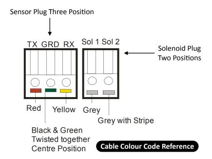
The Water Witch's designed to be installed close to the pool equipment. Both the sensor and solenoid leads are normally 5 meters long with plugs attached for connection to the base of the control box as shown. (Water Witch 20 & 30 for Balance Tank installs come with 20 & 30 meter Sensor lead respectively).
